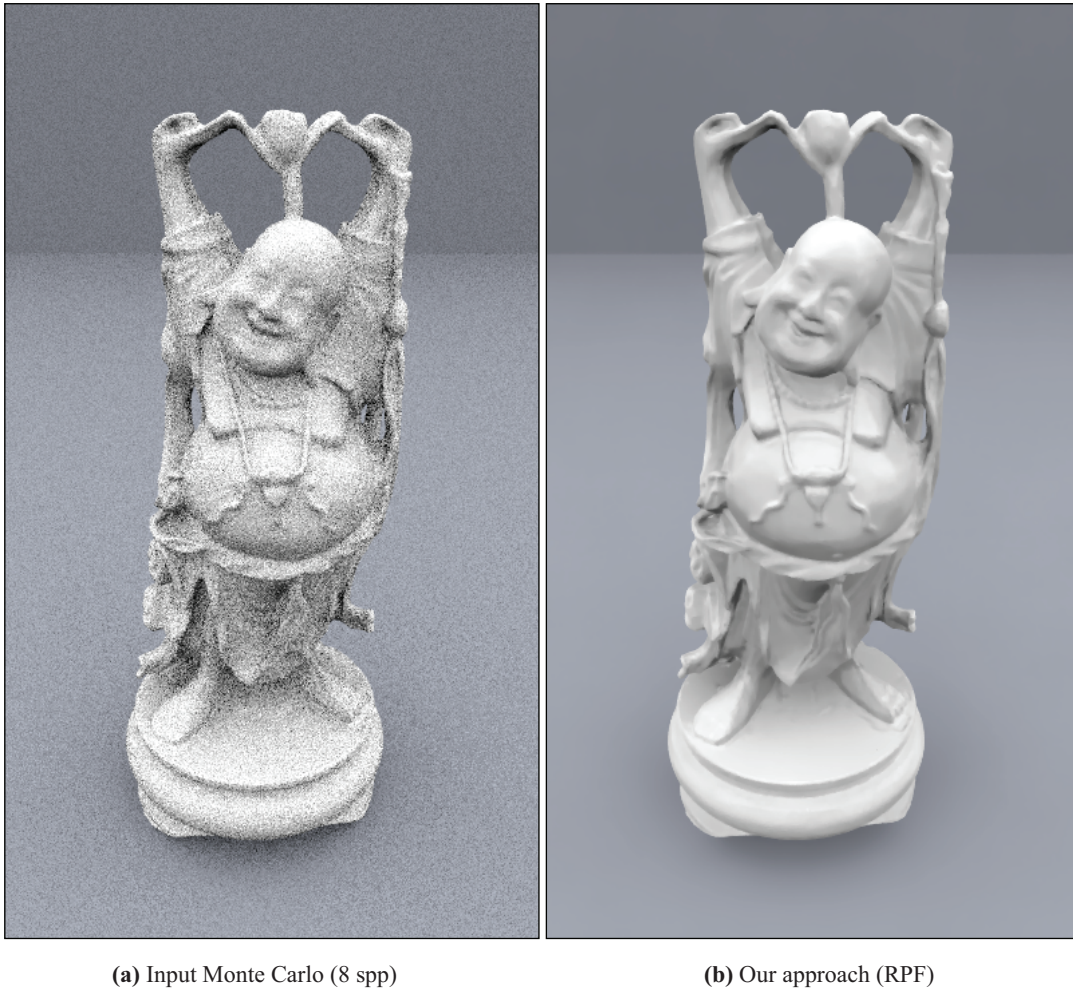
Fig. 8. Here, the simple BUDDHA model is illuminated by a disk area light source. Our algorithm is able to remove the random noise from the area light source but keeps the geometrical detail in the Buddha statue.
