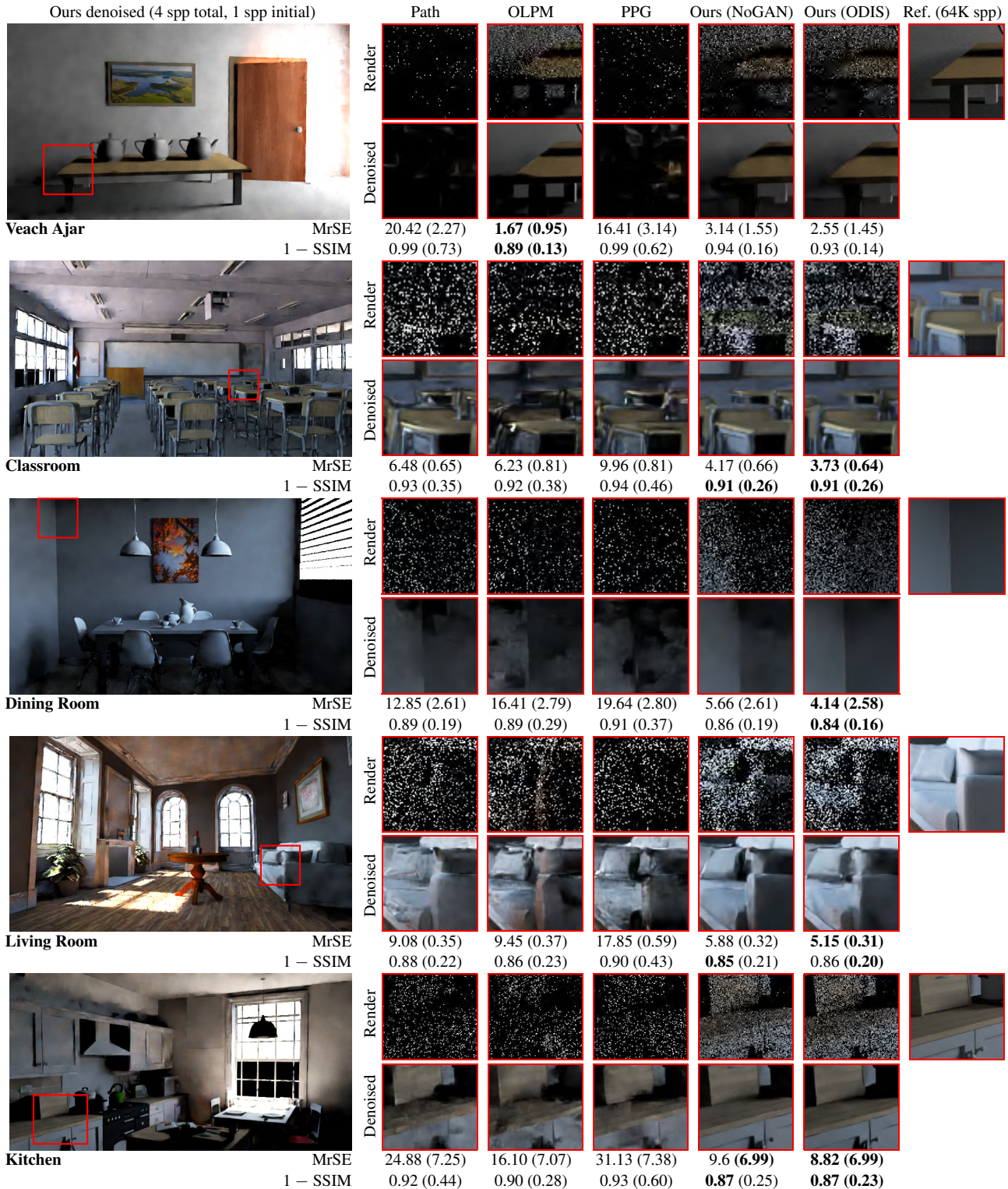
Figure 8: Equal-sample comparisons with state-of-the-art importance sampling techniques in Mitsuba including OLPM [VKv*14] and PPG [MGN17]. The top row shows the rendered output using the sampling technique, while the bottom row demonstrates the results of also applying KPCN [BVM*17], an off-the-shelf MC denoiser. Both MrSE and 1-SSIM are reported below for the rendered output and the denoised result (in parentheses). Ours and Ours (NoGAN) are relatively more converged, which significantly improves the final denoised output. Although the NoGAN version outperforms previous methods, there are still regions where it underperforms relative to our full algorithm. Our networks were trained with Blender/Cycles scenes and were not retrained for Mitsuba. Full images are in the supplemental.
