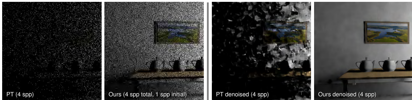
Figure 1: We propose an offline, deep-learning approach to importance sample and improve convergence of path traced images, especially at low sample counts. The two leftmost images are results comparing standard path tracing (PT) to sampling using our neural network at 4 samples per pixel (spp) on a test scene in Mitsuba [Jak10]. Here, our network is given only an initial 1 spp as input to generate a sampling map that guides the remaining 3 spp. Unlike existing learning-based path-guiding methods, our network is used only in inference mode for test scenes and does not require any retraining or optimization per scene. Our system focuses on faster convergence for low sample counts in order to improve performance of post-process applications, such as Monte Carlo (MC) denoisers. On the right, we show how our method can be coupled with an off-the-shelf MC denoiser [BVM*17] to get better results.
